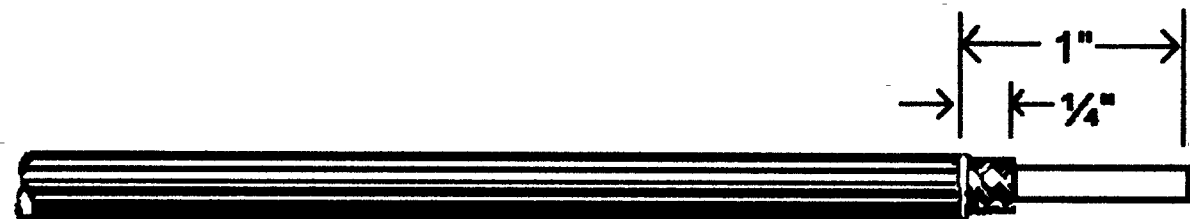
Figure 4 - Coax cable preparation. The \frac{1}{4} " braid length is approximate and can be longer - it will be trimmed later.
