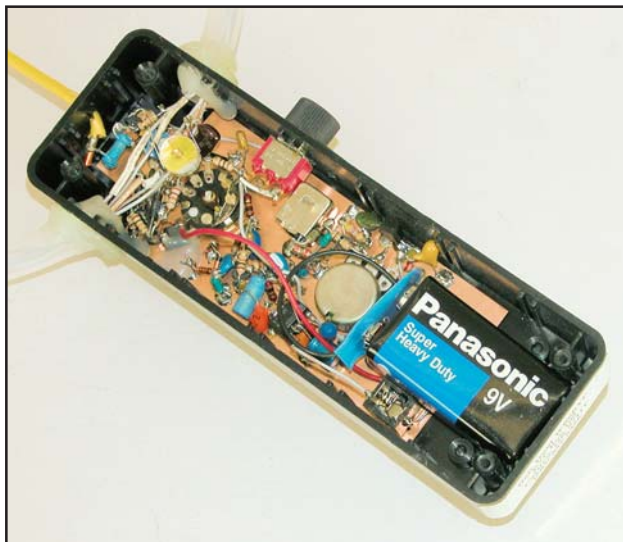
Figure 4—This early prototype of the 80-meter DF receiver uses a Radio Shack 270-1804 plastic case and “ugly construction.” The RF gain control can be operated with the thumb and the sense antenna switch with the index finger. The sense antenna circuit (Q5) is at the top, the RF amp (Q1 and Q2) is under the loop wiring and C14. T1 is secured with a drop of hot melt glue just left of R4. L4 is in the rectangular metal can just below S1, with Q3 just below it. U1 is on the left side just above the tuning control, R12. The headphone jack is beside the battery, and the plastic tubing for the loop antenna is glued to the case. The yellow wire for the sense antenna protrudes from the top.
